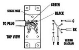
Figure 8—The drawing on the left shows the encoder housing and wires coming from the plug. The diagram to the right shows a schematic of where each wire is connected. Swapping the black and green wires will change the + and - directions of the readout.
