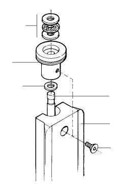
when the screws are tightened, you can remove the housing shell and sand the mating surfaces on a piece of sandpaper on a flat surface until they grip the collar tightly enough.
