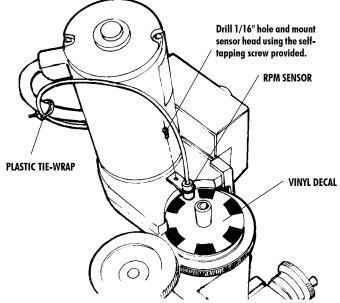
FIGURE 7—Mounting the sensor to the belt housing
