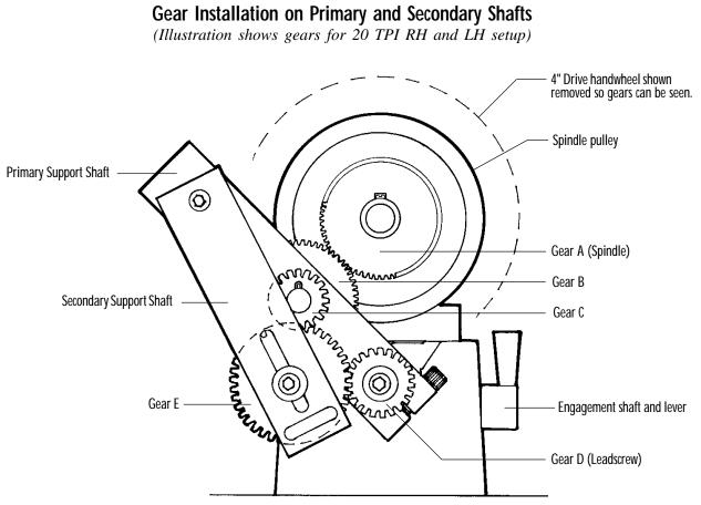
Figure 7a—Gears A, B, C, D and E installed for cutting a right-hand thread
