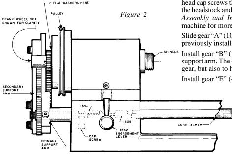
Side view, thread cutting attachment installed
