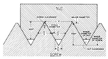
Figure 1—Component parts of a thread cut with a sharp pointed 60° Vee tool.
