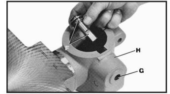
3. Insert shaft of worm gear (F) Fig. 4, into hole (G) from inside of table bracket (H).
