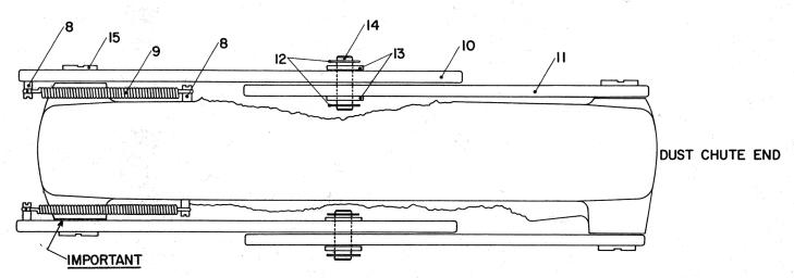
DUE TO VARIATION IN THE GUARD CASTINGS IT MAY BE NECESSARY TO ADD ONE 904-01-031-7712 WASHER BETWEEN REAR LEAF GUARD AND LEFT REAR BOSS ON GUARD CASTINGS.
