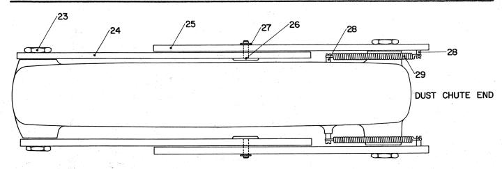
NOTE LOCATION OF SPRING STUDS AND RELATIONSHIP OF FRONT AND REAR LEAF GUARD HALVES
