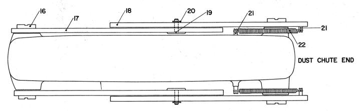
NOTE LOCATION OF SPRING STUDS AND RELATIONSHIP OF FRONT AND REAR LEAF GUARD HALVES
