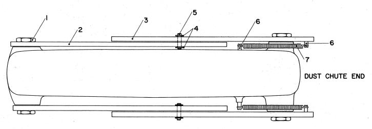
NOTE LOCATION OF SPRING STUDS AND RELATIONSHIP OF FRONT AND REAR LEAF GUARD HALVES
