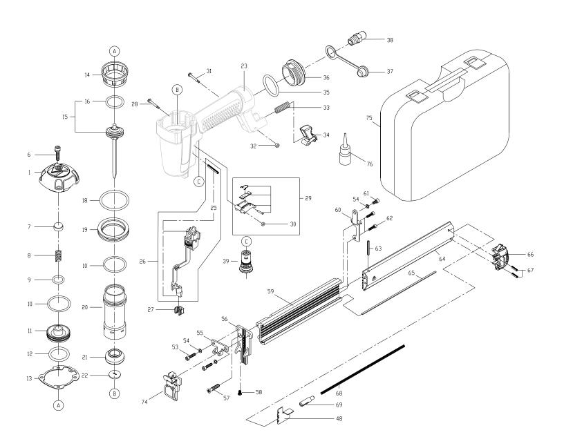
NOTE: PARTS LIGHTLY SHADED ARE NOT SERVICEABLE.
