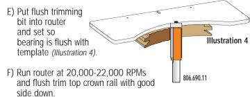
NOTE: WHEN STARTING CUT, ALWAYS REMEMBER TO MAKE CONTACT WITH BEARING TO A PLACE ON THE TEMPLATE WHERE THERE IS NO WOOD TO PREVENT KICKBACK.
