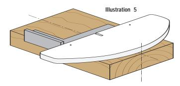
**NOTE:** DRIVE NAILS IN ABOUT 1/4"-3/8". THE NAIL HOLES WILL BE MACHINED OUT WHEN RAISED PANEL CUT IS MADE.
