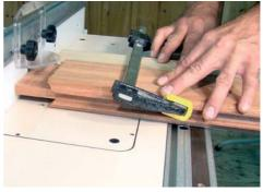
Cut the extra-long tenons by moving the fence back from the cutter and undercutting the tenon produced in the previous steps.
