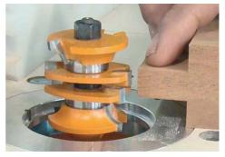
Insert the long grain cutter in the router table. Set the height of the cutter so the top of the cutter is even with the top of the tenon you made previously.
