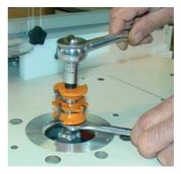
Slide the upper slot cutter back on to the arbor, making sure the carbide tips are clear of each other. Replace the bearing and upper cutter. Store the two spacers you removed in the previous step between the upper cutter and nut. Tighten the bit stack.
