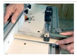
As before, use the Gauge Stick to make the fence parallel to and the correct distance from the miter gauge slot.
