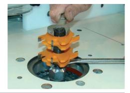
Set aside the three upper slot cutters and remove the spacers from between two cutter sets.
