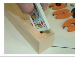
Use the same stack of cards to determine which spacers should be placed between the cutter sets.
