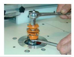
Slide the top cutter, bearing, and upper slot cutter off the bit arbor. Remove the two spacers from between the upper and lower slot cutters.
