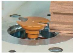
Set the height so it's even with the groove produced in the previous step.
