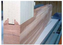
If the fence is too far back the tenon will be too long, as shown here. In this case move both ends of the fence forward.
