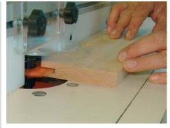
Position the fence to control the depth of the slot. Make the slotting cut.
