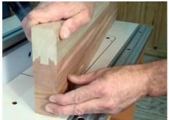
The positive profile formed on the edge of the support block will fit into the negative profile of the long grain cut.
