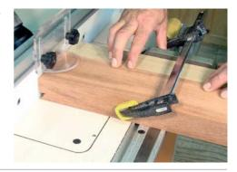
Clamp the square edge of the support block against the material when the trailing edge is square. Machine both ends of all the rails.
