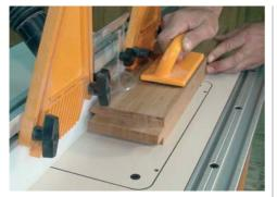
Make a test cut in a piece of scrap that is the same thickness as your door material. Featherboards on the fence will help hold the material down to the router table top.
