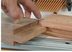
Check the set up by slipping a tenon into the groove and checking alignment across the tops of the pieces. The tops of both pieces should be even. Adjust the height of the bit as needed.
