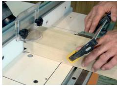
Make a test cut and check the set up. Machine a test piece
