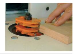
Make a test cut. Use a piece of scrap behind the rail to prevent blowout when the bit exits. Narrow pieces must be clamped into a miter gauge.
