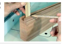
Align the mark on the Gauge Stick with the tip of the coping cutter and clamp the Gauge Stick to the miter gauge.
