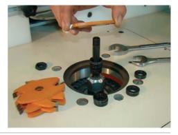
Tighten the bit stack.
