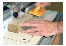
Machine a support block when the fence position and cutter height are correct. The support block must be the same thickness as your door material, 2-1/2-in. wide and 16-in. long.
