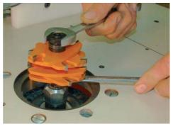
Replace the upper set of cutters and tighten the bit stack.
