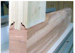
If the fence is too far forward the tenon will be too short, as shown here. Adjust the fence by moving both ends.
