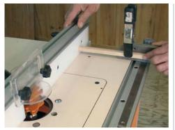
As before, use the Gauge Stick to set the fence parallel to the miter gauge slot.
