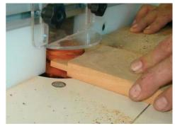
After accurately machining the tenon, cut the shoulders on the top and bottom by standing the board on edge.
