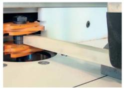
After the preliminary cuts are made you're ready for the full depth pass. Touch the Gauge Stick against the core of the tenon cutter while clamping the stick to the miter gauge.
