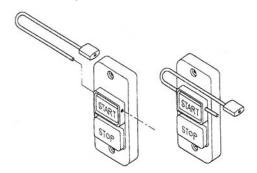
Figure 20: Switch Lock Out
