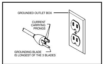
Repair or replace damaged or worn cord immediately.
