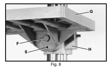
9. Assemble table (G) Fig. 8, to table bracket (H) using bolt (F). Line up hole (S) in table with hole in table bracket and insert pin (P) Fig. 9.
