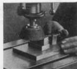
Surface grinding on the drill press, using a cup wheel on the No. 991 spindle.
