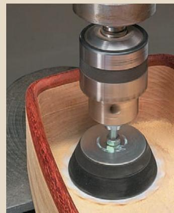
A Tim Skilton Sanding Pad attached to your drill press works great for smoothing out the bottom and curved inner surfaces of the bowl.
