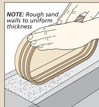
**Shaping the Walls.** A belt sander will quickly shape the walls to the desired thickness.
